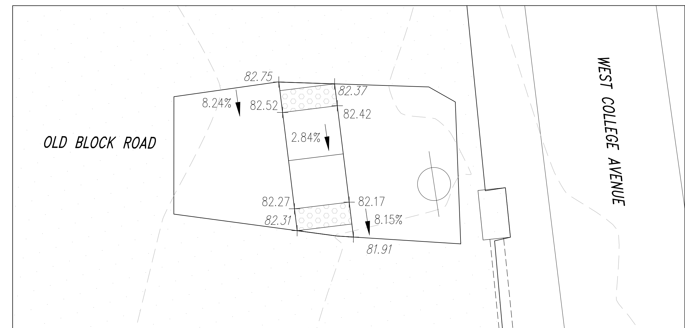
CURB RAMP DETAIL SCALE: 1"=5'
