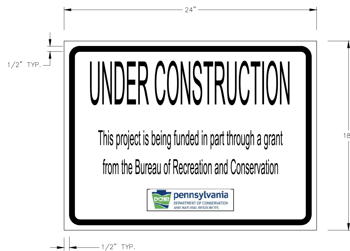
TEMPORARY UNDER CONSTRUCTION SIGN NOT TO SCALE
