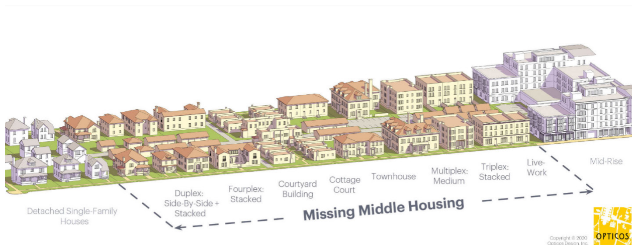
FIGURE 11 EXAMPLE OF MISSING MIDDLE HOUSING TYPES
