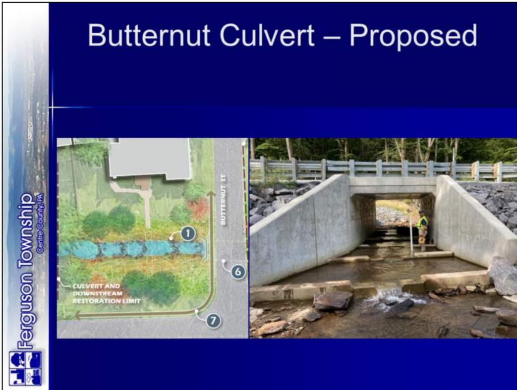
If the township wishes to pursue the design and permitting for this project, we would propose to replace the culvert with a depressed concrete box culvert, with Step pools downstream of the culvert to tie into the existing grade downstream of the vertical drop.
