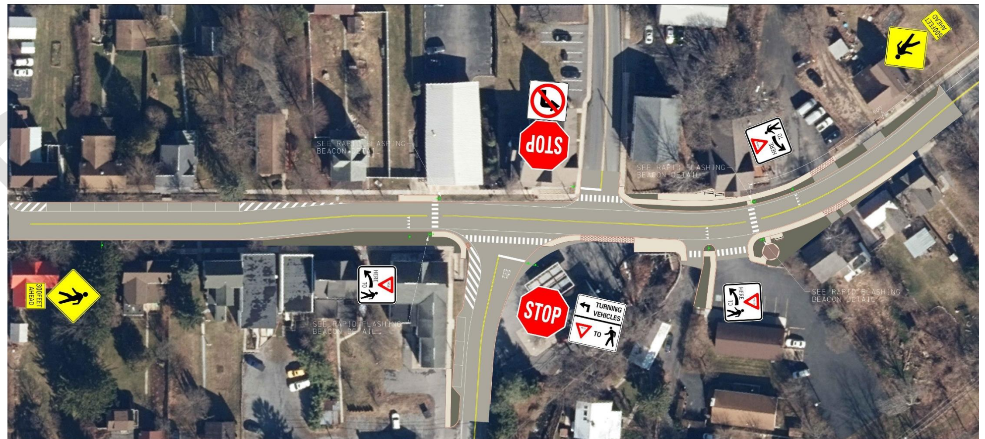
Figure 14. Pine Grove Road & Water Street/Nixon Road – Concept A.1, Stop Controlled Option
