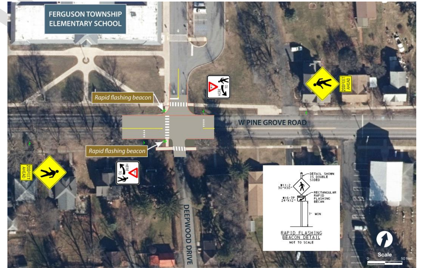
Figure 25. Concept C.4, Pine Grove Road Enhanced Crossing at Deepwood Drive (East)
