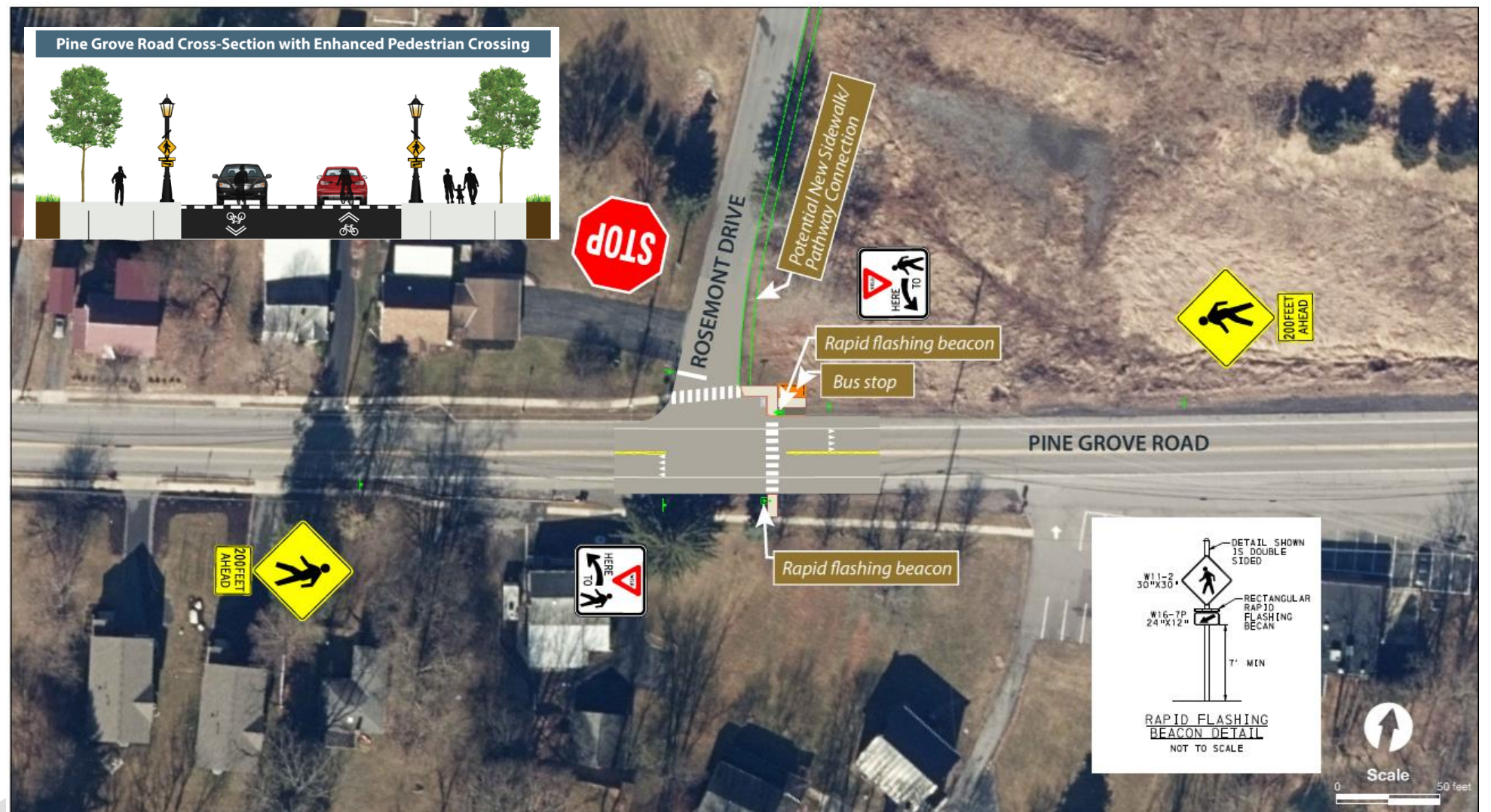
Figure 23. Concept C.2, Pine Grove Road Enhanced Crossing at Rosemont Drive
