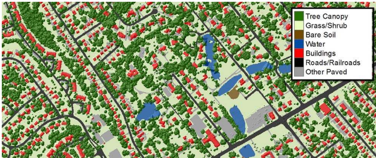
Figure 4 - A sample of seven class high-resolution land cover developed by our team using the USDA Forest Service tree canopy assessment protocols.
