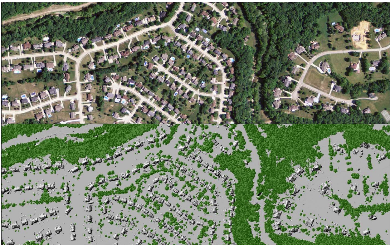
Figure 3 - An example of a tree canopy mapping project carried out by our team for a multi-county region in which leaf-on imagery (top) and leaf-off LiDAR (bottom), acquired in different years were used to accurately extract tree canopy (bottom).
