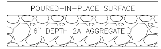
POURED-IN-PLACE FALL SURFACE ALT #2 NOT TO SCALE
