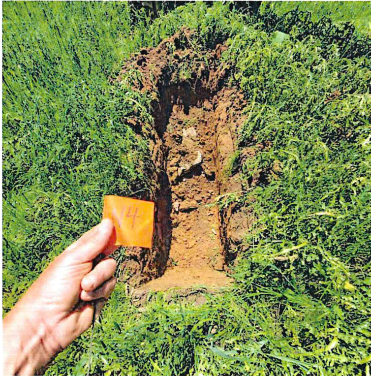
Photograph 12: Thin alluvium in test pit N1 (only 2' of "presumed" alluvium)
