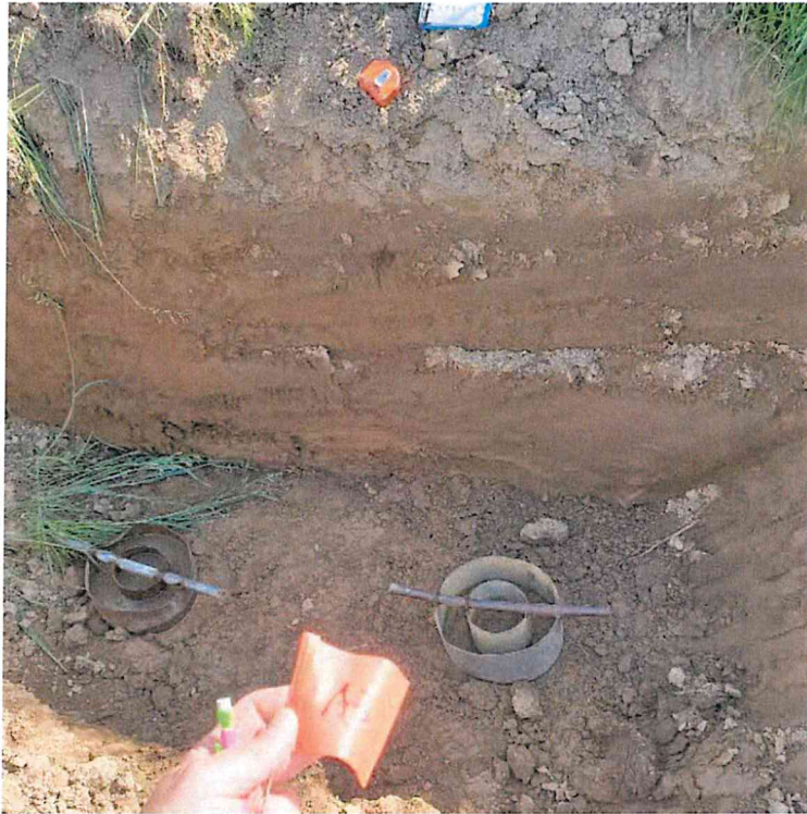
Photograph 6: Infiltrometer testing of "presumed" alluvial Bw 3 -horizon at test pit A2
