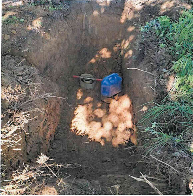
Photograph 10: Non-Conventional infiltration testing in test pit C1
