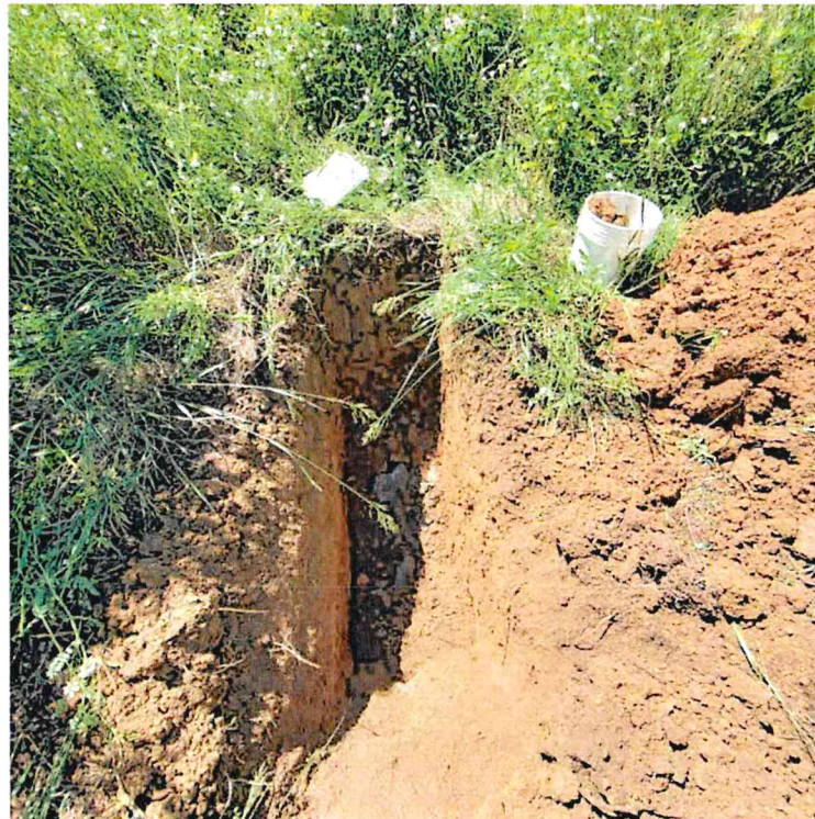
Photograph 12: Thin alluvium in test pit N1 (only 2' of "presumed" alluvium)
