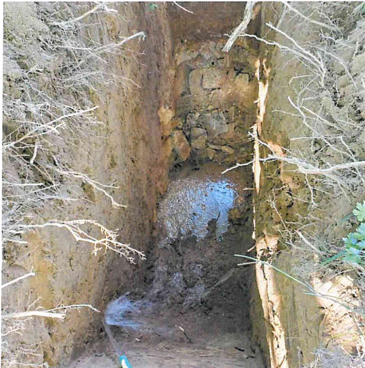
Photograph 10: Non-Conventional infiltration testing in test pit C1
