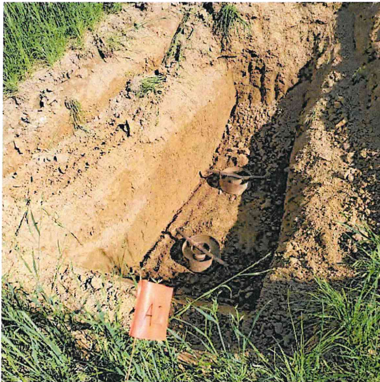
Photograph 6: Infiltrometer testing of "presumed" alluvial Bw 3 -horizon at test pit A2
