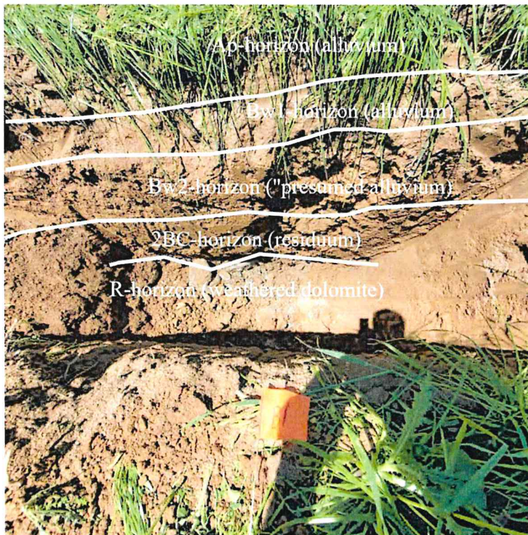
Photograph 4: Non-distinct boundaries between alluvium, residuum, and weathered rock (B1)
